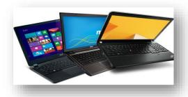
Metals (aluminum, steel), glass, plastics and (rare) metals like gold, cobalt, lead, silver and indium. The wiring consists of copper ad plastics.
